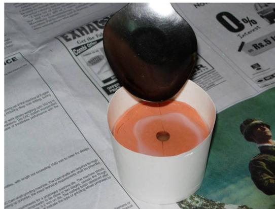
Fig 6: Mould filled with wax
