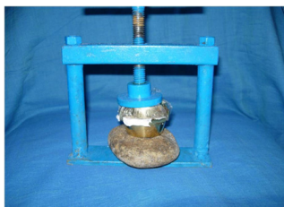
Fig 11b: Heat Cure Resin Packed
